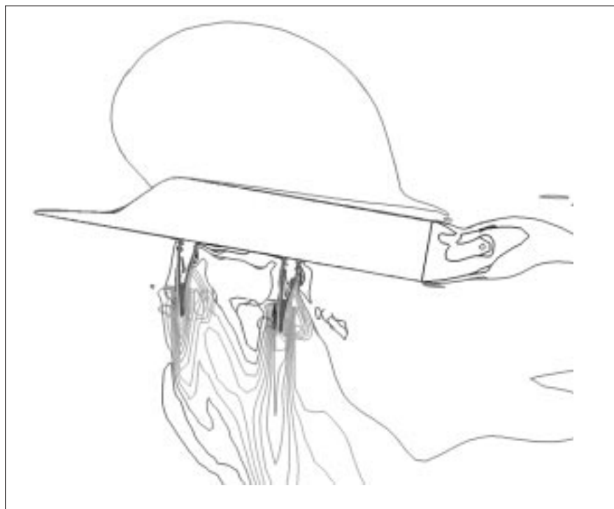
Fig. 1. Mach number contours taken in the symmetry plane to illustrate the deflection of lift jets.
