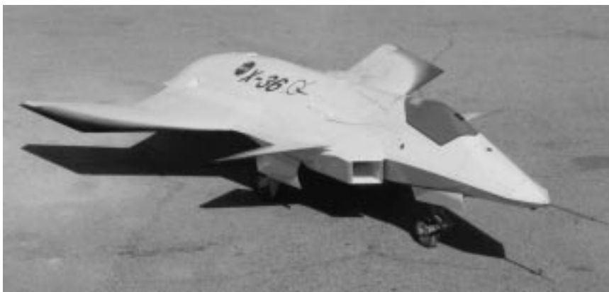
Fig. 1. X-36 Tailless Fighter Agility Research Aircraft prepares for flight at the Dryden Flight Research Center.
