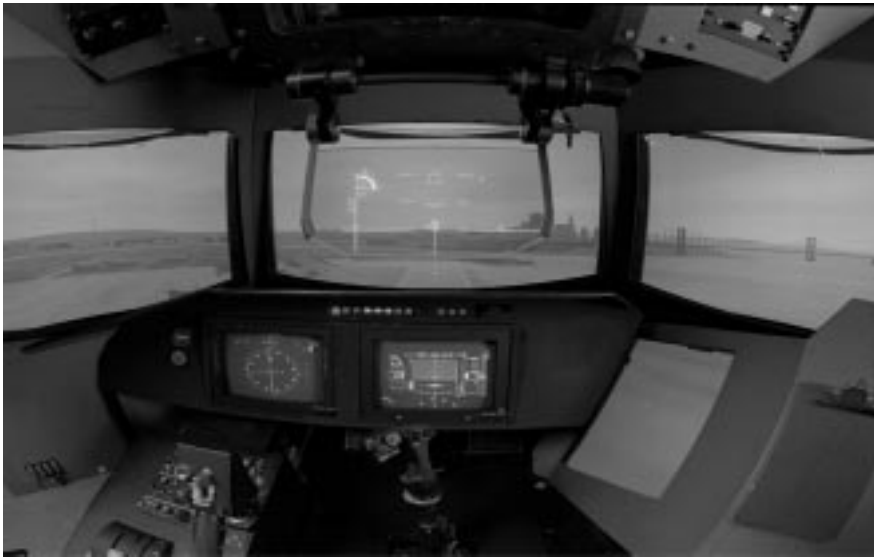
Fig. 2. Pilot's view on approach to urban vertiport. Electronic cockpit displays provide guidance for complex noise-abatement approach profiles.
