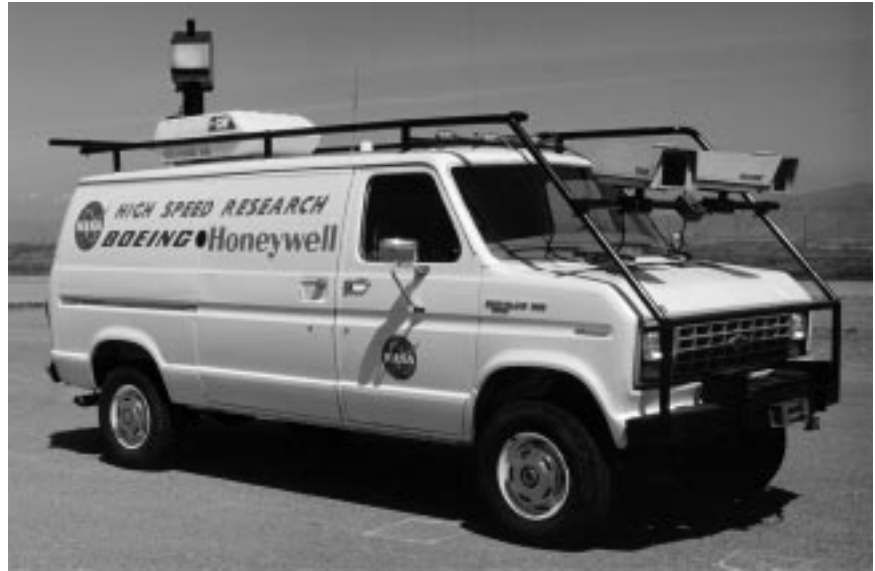
Fig. 1. The SOREV. Externally mounted cameras feed the forward and inboard displays at the rear driver station. An outboard side window is configured to simulate the side window visibility planned for the HSCT.
